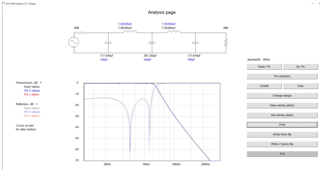
Picture 6: Filter design Tschebyscheff - Lowpass 6MHz (L1, L2, C1...C4)
