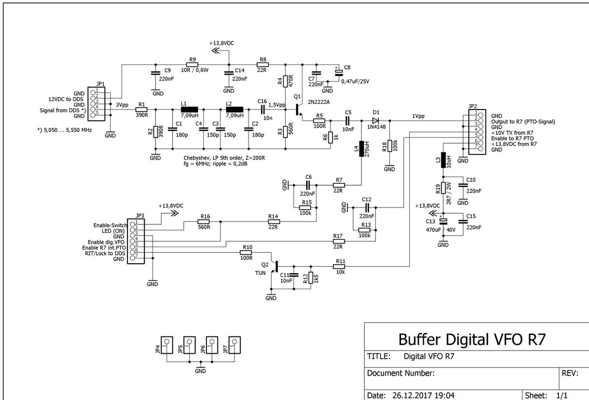
Picture 4: Buffer schematic
