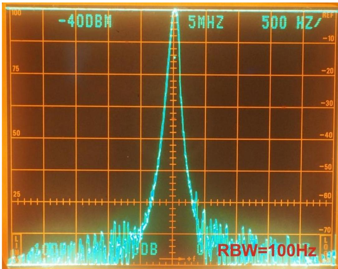
Picture 10: Spectra of 7-line PTO and digital VFO
