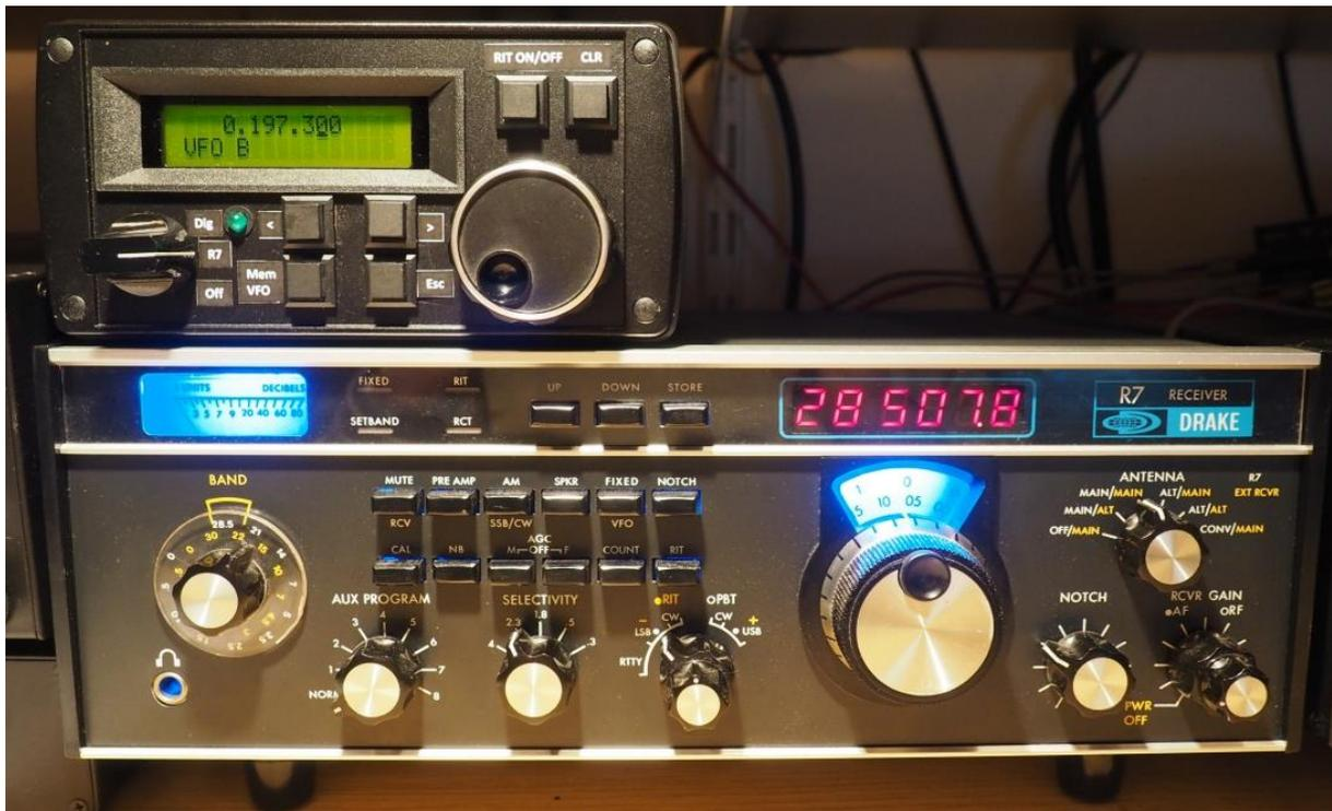
Picture 15: Dig. VFO B operates but doesn't control the R7
