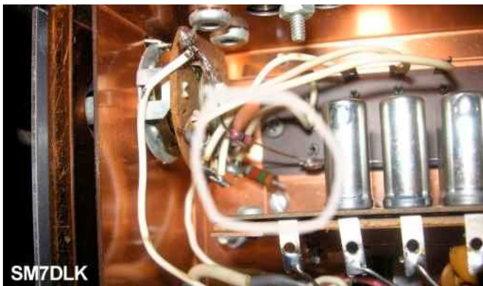
Picture 21: T-4XB, cut resistor
