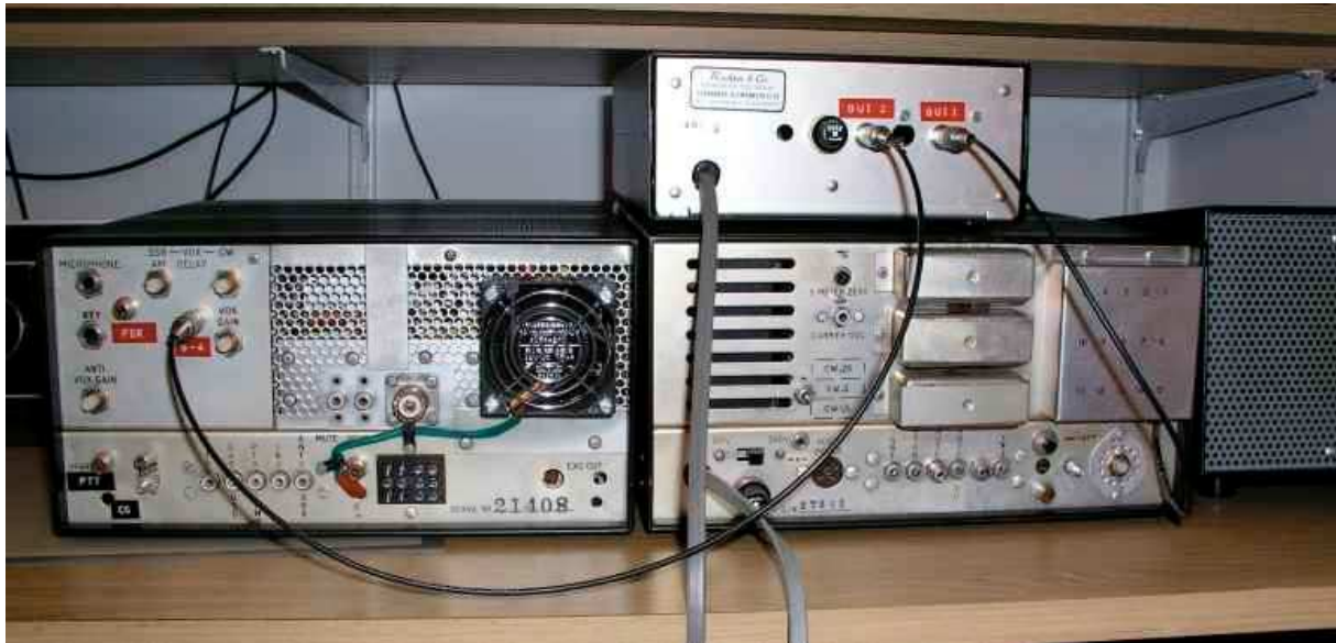
Picture 16: Rear side of the FS-4, R-4C and T-4XC with cabling
