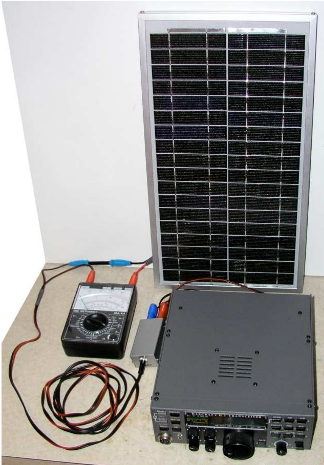
Picture 4: K2-Charger with solar cell, multimeter (Ammeter) and K2
