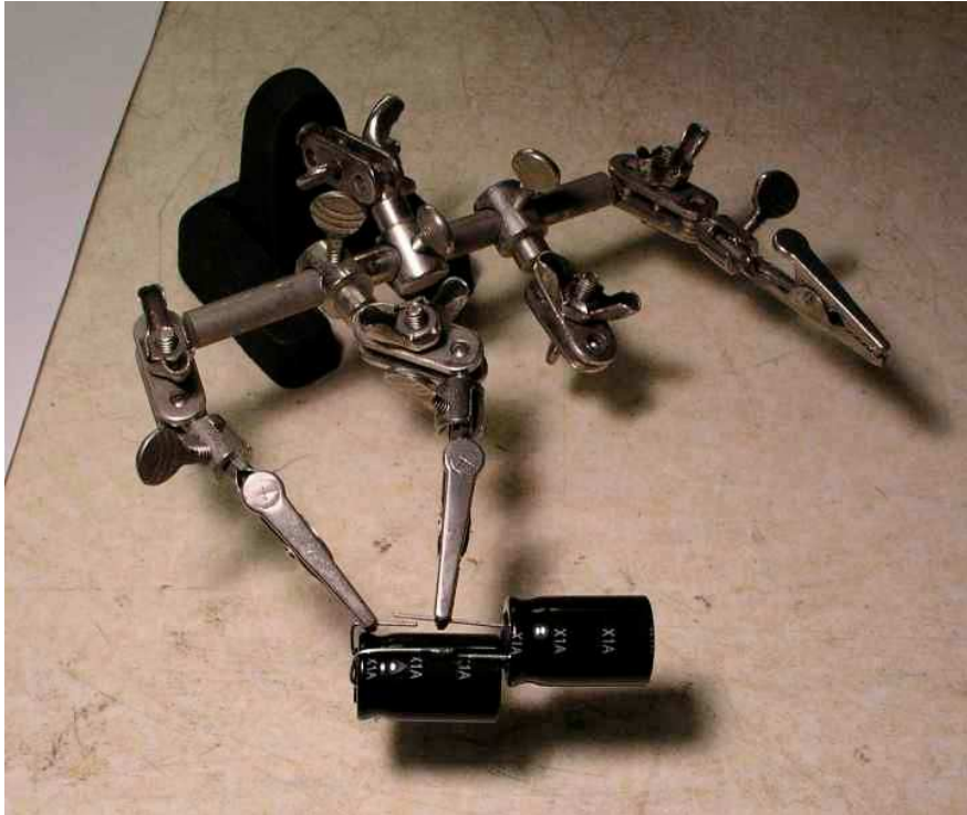
Picture 7: Soldering of the new cap's with „helping hand“
