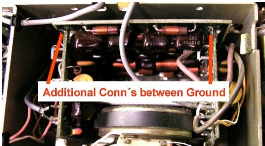
**Picture 4: Additional groundconnections in the highpassmodule**
