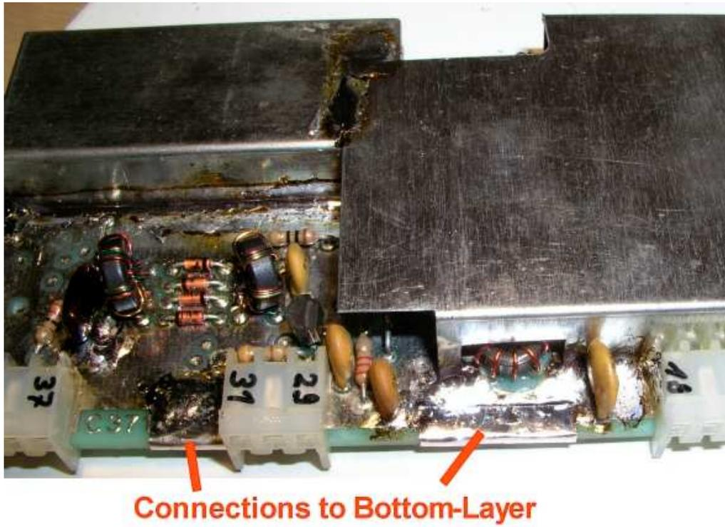
Picture 10: Connections between top- / bottomlayer
