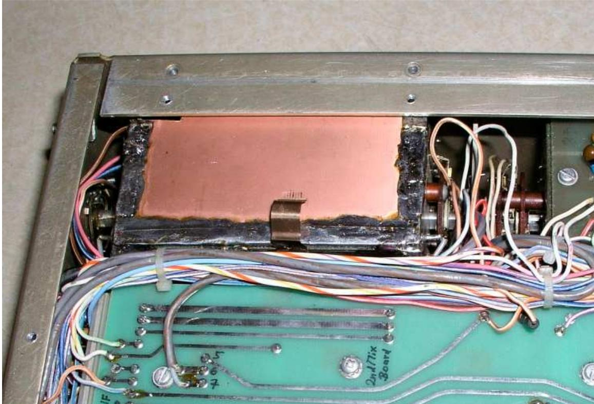
**Picture 13: Shield for the lowpassmodule – lower side**
