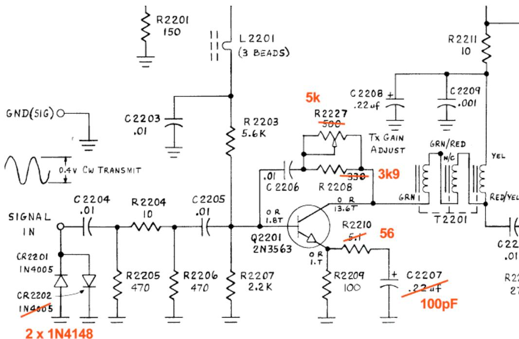
**Picture 3: Increasing the predriver's input impedance (old version with 3 transistors)**
