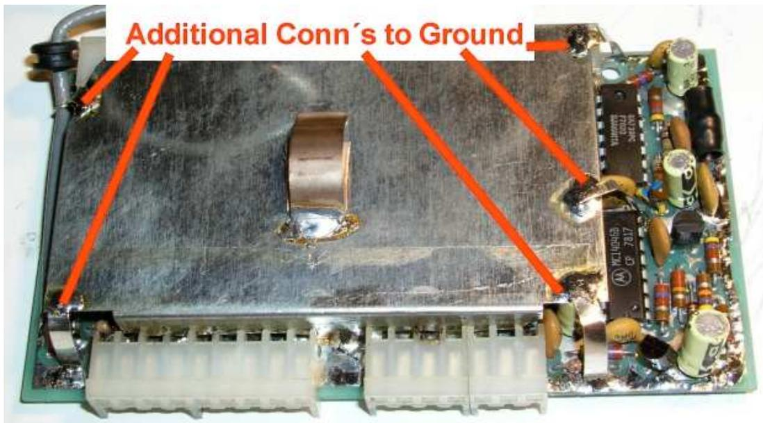
Picture 11: Shielding used as additional ground-layer
