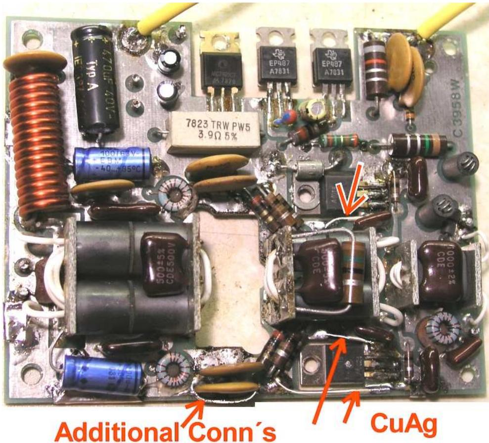
**Picture 2: Additional connections in the groundplane (PA)**
