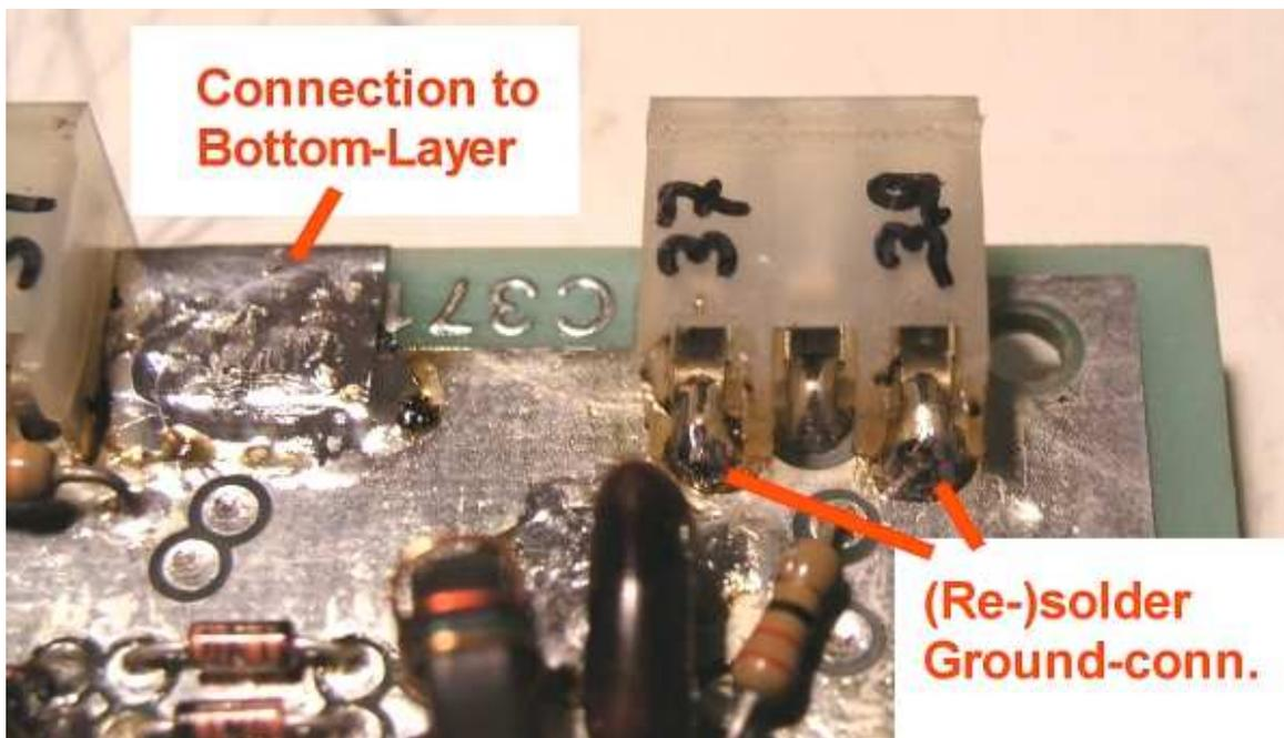
Picture 9: Resoldered connectors and connections top- / bottomlayer
