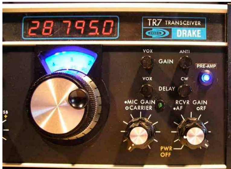
Picture 4: Blue ON/OFF-switch and label at the TR7's frontpanel (right side)
